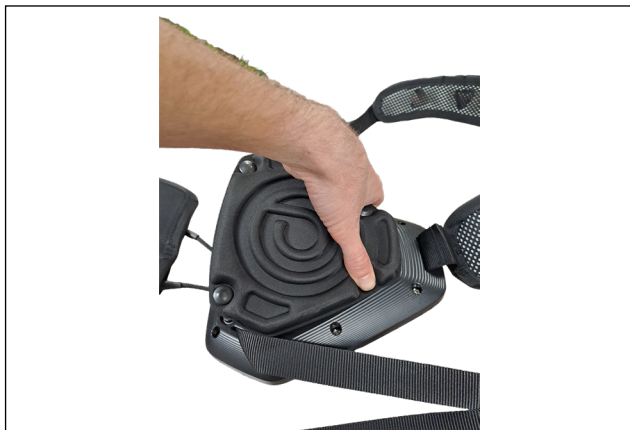
Figure 33a et 33b: Reassembly of the fabric pad (Step 4)
