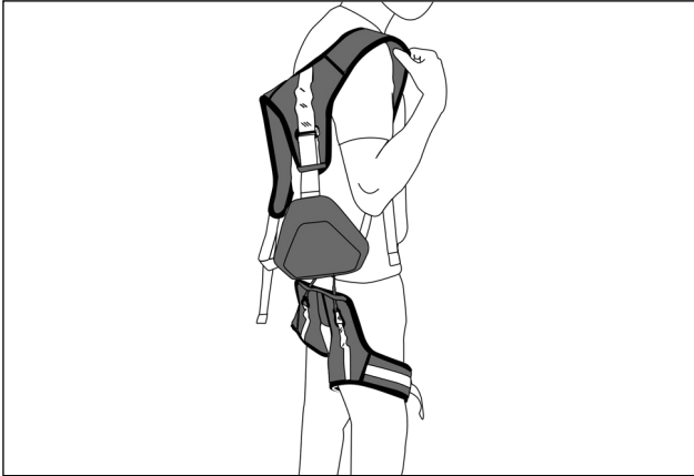
Figures 9a and 9b: Putting on the shoulder straps (Step 4)
